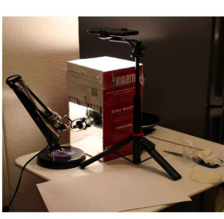
The photography arrangement for identifying cheese clumps in the sauce, which stood out as dark blotches in the photographs taken with the tripod-mounted iPhone. Martina Gaiba
