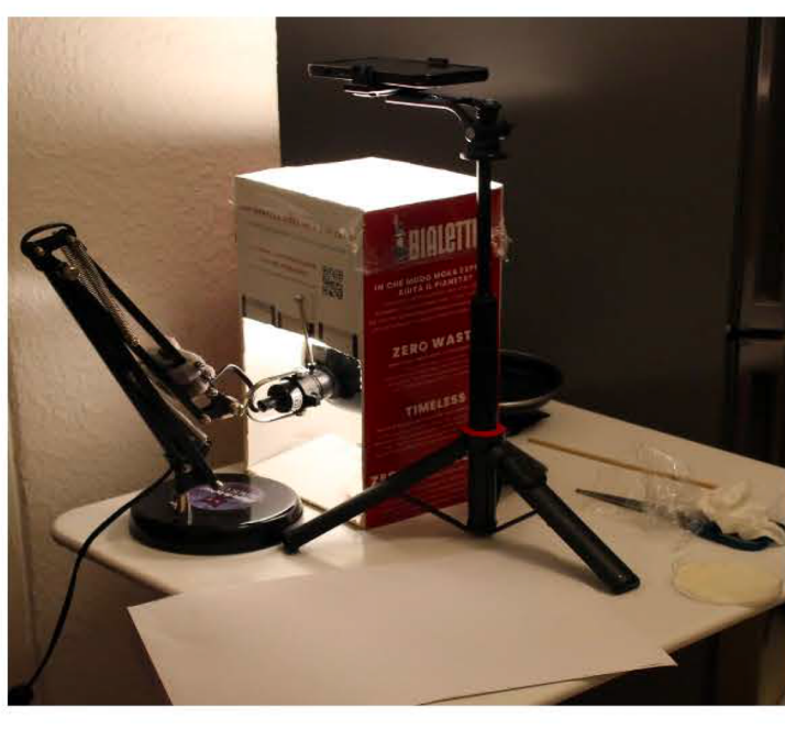
The photography arrangement for identifying cheese clumps in the sauce, which stood out as dark blotches in the photographs taken with the tripod-mounted iPhone. Martina Gaiba
